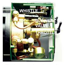
It will take approximately 7 minutes to raise pressure. Once the gauge reaches 20 lbs, you can shut off and remove suction fan from the stack and then turn on the engines internal blower. At this point steam will rise rapidly!
